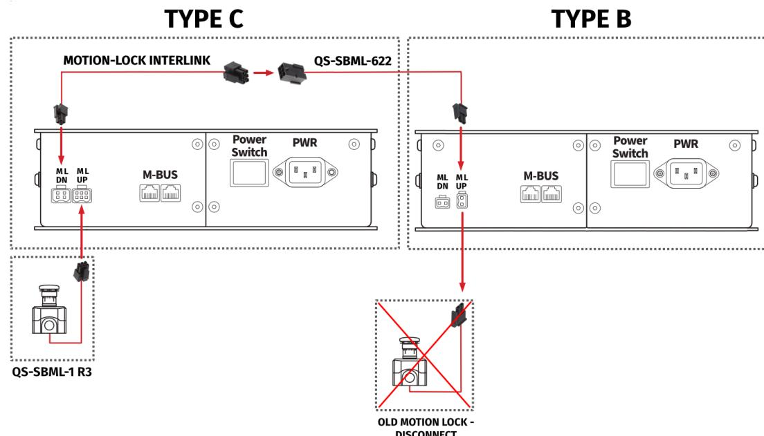
Adapter can be used to connect TYPE B Power Cabinet directly with Motion Lock (QS-SBML-1 R3):
