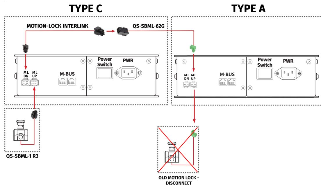
Adapter can be used to connect TYPE A Power Cabinet directly with Motion Lock (QS-SBML-1 R3):
